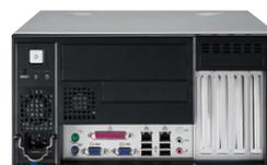
Plug ring-lock securely fastens the power cord
